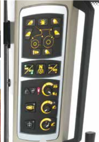
Pillar mounted PTO speed selection controls and linkage controls.
